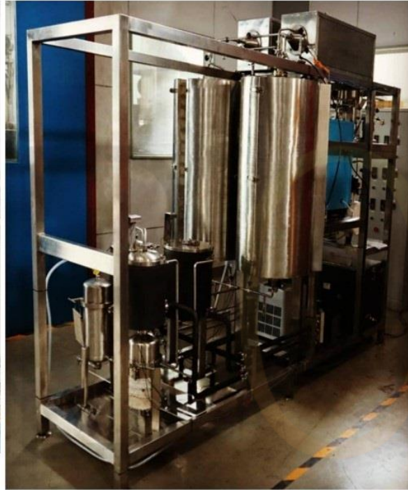
Bench-scale unit, 650 ml biogasoline/hr.
